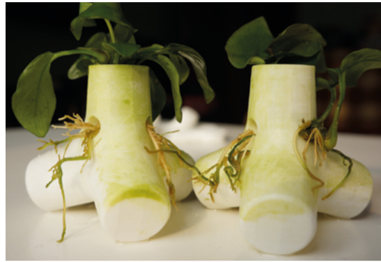
THE TETRAPOT IS A CONCRETE SEA DEFENCE HOLLOW ELEMENT CONTAINING MANGROVE AND OTHER PLANTS SEEDS, WITH THE AIM TO COMBAT THE DEFORESTATION OF COASTLINES.
